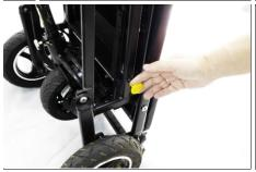
Locate small yellow toggle on side and pull to release front wheel assembly.
