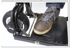
...if not press your foot down onto the footplate to lock the scooter open.
