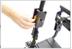
Press and hold the small yellow latch on the steering column...
