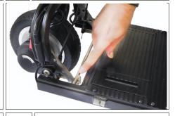
Make sure the locking latches have locked to the steel bar...
