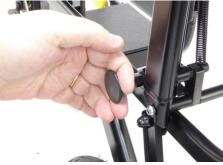
If the scooter has armrests pull the black toggle to release then fold backrest down as per (1)
