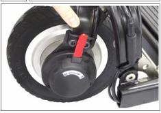
Check that the magnetic brake is in the LOCKED position to engage the motor.
