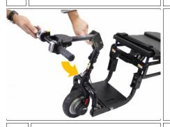
...and fold the column down until it is locked by the magnetic catch.
