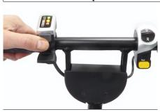
To turn the scooter on press the grey button below the battery display.
