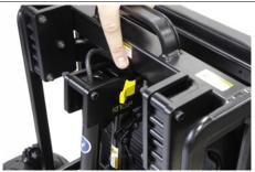
Press in steering column to lock it tightly against the frame.
