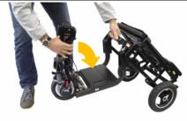
Firmly hold the scooter by its steering column and the carry handle and firmly press the column down towards the footplate
