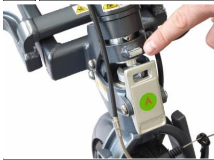
10 ...and make sure the column key locks into place under latch 'A'.
