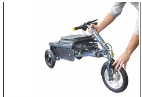
9 Pull the steering column upright...
