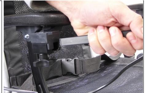
**4** Install armrest supports into the slots and press them down until they lock. Keep cables away from pinch points
