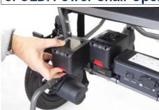
Batteries can be removed by pressing the red tab upwards and pulling backwards.
