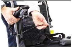
Keep controller cable away from pinch points like the armrest supports.
