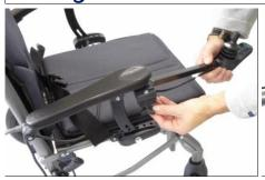
Slightly loosen the knurled knob and remove the controller.
