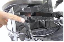
adjust the position of the controller and tighten with the knurled knob.
