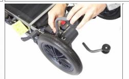
Install the anti-tip wheels if desired. These simply press and lock into place
